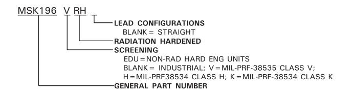
The above example is a Class V screened device with straight leads.
